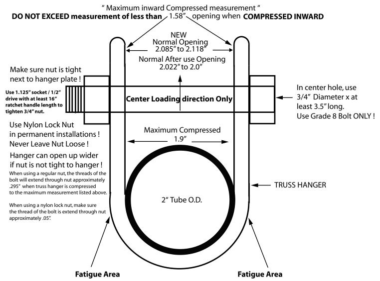
When using one 5/8" shackle ONLY on either side of Truss Hanger!
